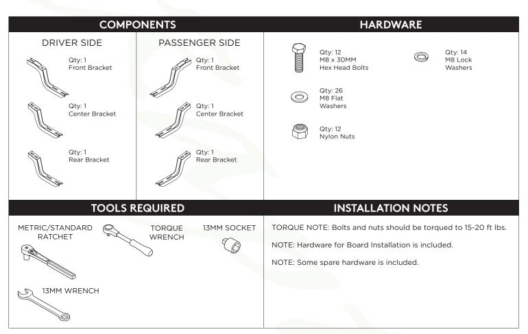
Remove all contents from the package and check brackets for any damage. Also, verify that all components and hardware listed above are included before you begin installation. If anything is missing or damaged please contact us at customerservice@raptorseries.com
