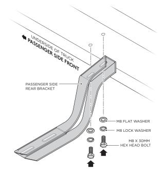
**3.** Fasten the top portion of the Passenger Side Center Bracket by using (2) M8 x 30MM Hex Head Bolts, (2) M8 Flat Washers and (2) M8 Lock Washers.
