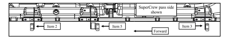
NOTE: (FOR SUPER CAB APPLICATIONS THE ORIENTATION OF BRACKETS ARE THE SAME. THE ONLY DIFFERENCE IS IT WILL NOT HAVE CENTER BRACKETS.)
