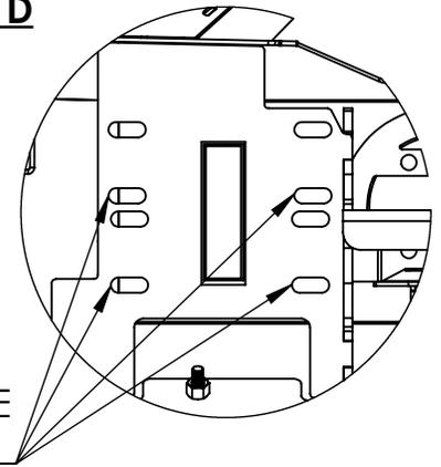
THESE HOLES ARE USED IF YOUR JEEP IS EQUIPPED WITH HILINE FENDERS.
