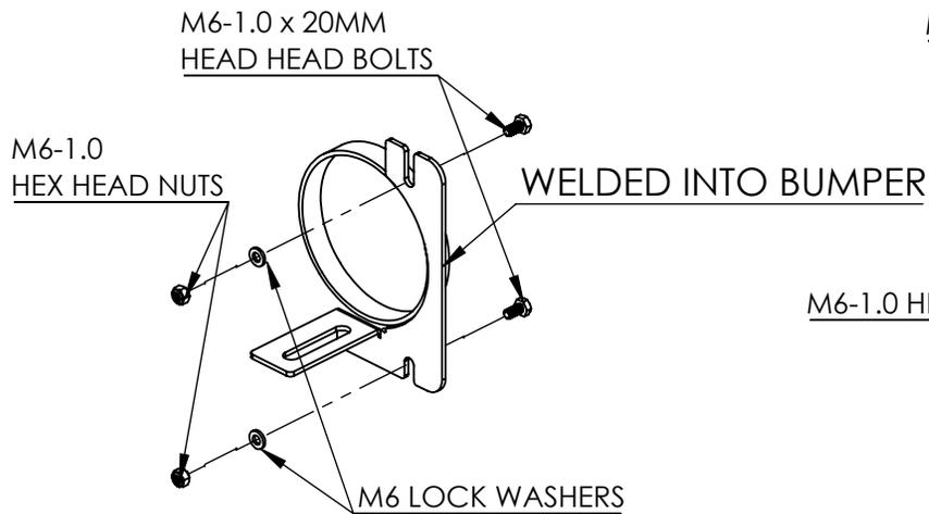
IF JL IS EQUIPPED WITH STEEL OEM BUMPER AND HAS THE VERTICAL STYLE OEM FOG LIGHT YOU WILL MOUNT FOG LIGHTS USING METHOD SHOWN IN FIG. A
