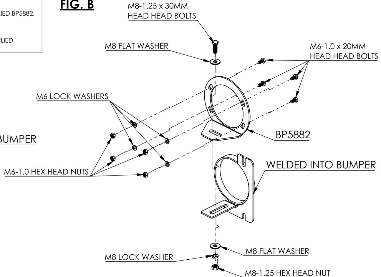
IF JL IS EQUIPPED WITH PLASTIC OEM BUMPER AND HAS THE JK STYLE OEM FOG LIGHT YOU WILL MOUNT FOG LIGHTS USING METHOD SHOWN IN FIG. B
