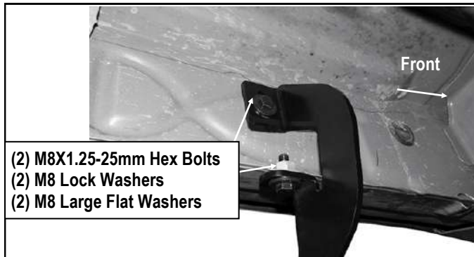
(Fig 6) Driver Side Front Bracket Installed
