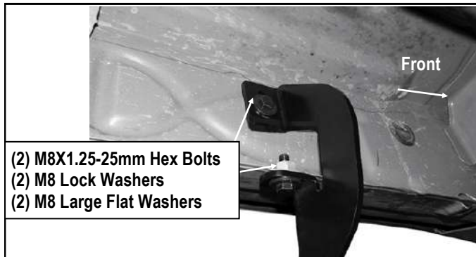
(Fig 6) Driver Side Front Bracket Installed
