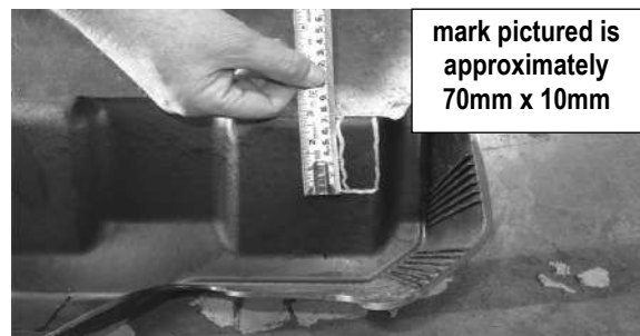
(Fig 14) 2017-On Passenger side DEF cover marked for trimming
