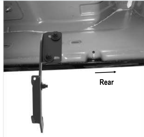
(Fig 10) Passenger Side Rear Brackets Installed
