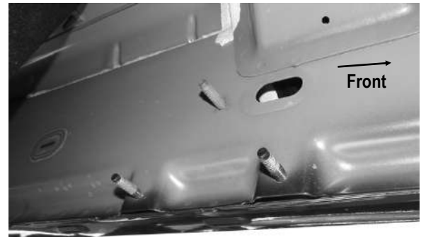
(Fig 3) Driver Center Mounting Bracket Location Pictured
