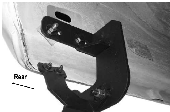
(Fig 12B) Driver Rear Brackets installed
