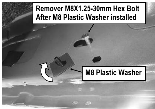
(Fig 5) Thread Plastic Washer Onto the Welded Bolt on M8 Bolt/Nut Plate To Hold Bolt/Nut Plate In Position. IMPORTANT: Do Not Remove The Hex Bolt Until The M8 Plastic Washer Has Been Threaded Onto the Welded Bolt.
