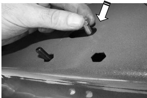
(Fig 4) Use The Loose Hex Bolt As A Handle. Insert The M8 Nut/Bolt Plate Into The Oval Hole And Feed The Threaded End Out Either Factory Hex Shaped Hole. IMPORTANT: Do Not Let Go Of The Hex Bolt Until After Plastic Retainer Has Been Threaded Onto Bolt (Fig 5)
