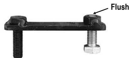
(Fig 3) Thread M8X1.25-30 Hex Bolt into the welded nut on the plate
