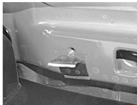
(Fig 2) Vehicle with 8mm Threaded Hole In Floor Panel
