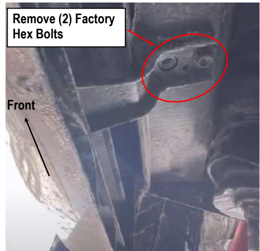
(Fig 5) Passenger Side Rear Mounting Location
