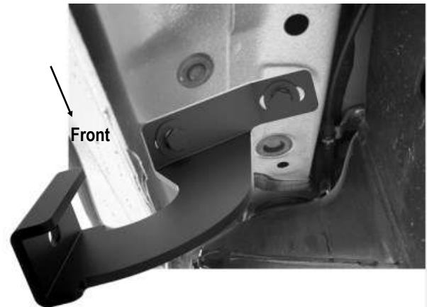
(Fig 4) Driver Front Mounting Bracket Installed
