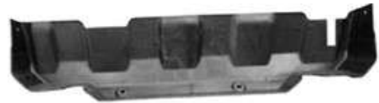
(Fig 17) 2017-Up Passenger Side DEF Cover Marked For Trimming
