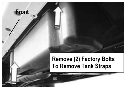
(Fig 12) Passenger side 07-16 DEF tank and cover
