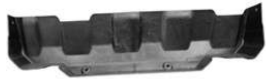
(Fig 13B) 17-on Passenger side DEF cover removed
