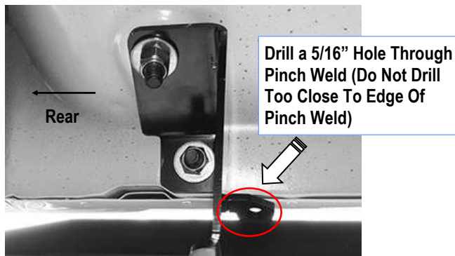
(Fig 10) Driver Hole On Driver Side Rear Mounting Location
