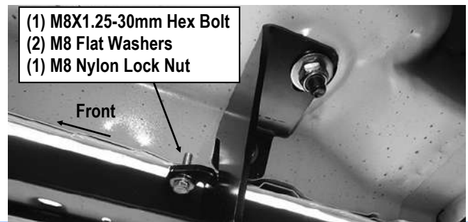
(Fig 19) Attach Passenger Center Mounting Bracket To Pinch Weld
