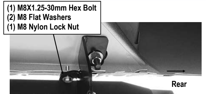
(Fig 21) Attach Passenger Rear Mounting Bracket (The Last One) to Pinch Weld
