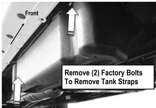
(Fig 14) 07-16 Passenger Side DEF Tank And Cover
