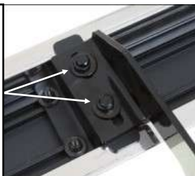
(Fig 11) Step Bar Installed on Bracket Installed (Example)
