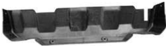
(Fig 18) 2017-Up Passenger Side DEF Cover Marked For Trimming
