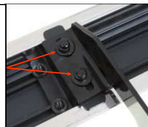
(Fig 13) Step Bar Installed on Bracket Installed (Example)
