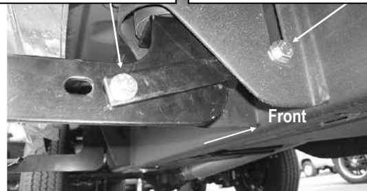
(Fig 6) Passenger Center Bracket Installed (1500 Models)
