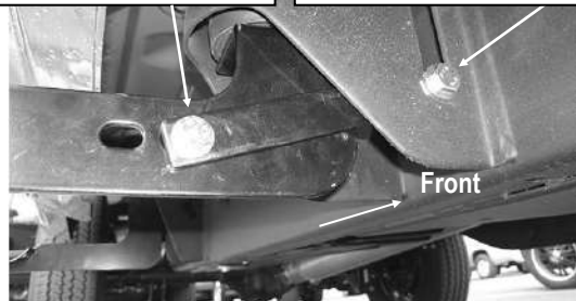
(Fig 6) Passenger Center Bracket Installed (1500 Models)
