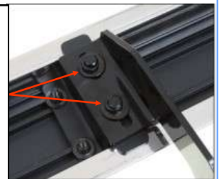
(Fig 12) Step Bar Installed on Bracket Installed (Example)
