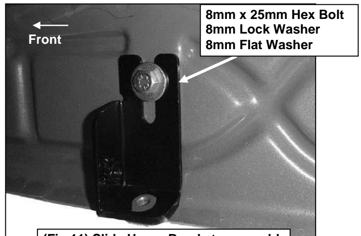
(Fig 11) Slide Upper Bracket over weld nut if equipped-also see Figure 2
