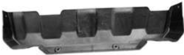
(Fig 13B) 2017 Passenger Side DEF Cover Removed
