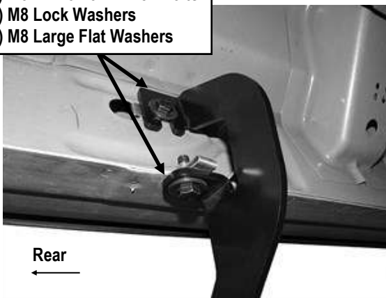
(Fig 8b) Assembled Driver Rear Mounting Bracket Installed
