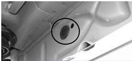
(Fig 4) Driver Side Center Mounting Location (With Rubber Plug on Mounting Hole)
