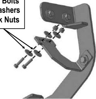
(Fig 10A) Attach Driver Front Support Bracket To the Back Of Pinch Weld (Models With Factory Holes In Pinch Weld Only)
