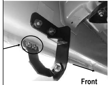
(Fig 10B) Driver Front Brackets installed
