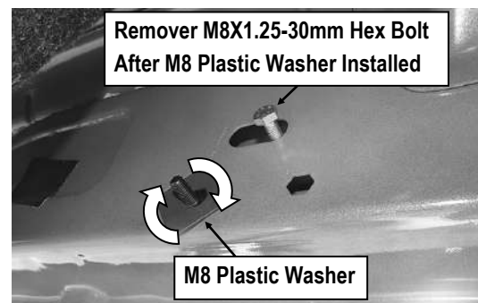
(Fig 5) Thread Plastic Washer Onto the Welded Bolt on M8 Bolt/Nut Plate To Hold Bolt/Nut Plate In Position. IMPORTANT: Do Not Remove The Hex Bolt Until The M8 Plastic Washer Has Been Threaded Onto the Welded Bolt.
