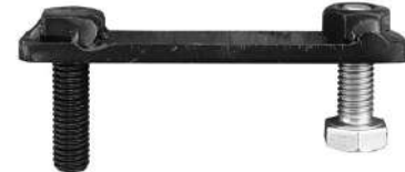
(Fig 3) Thread (1) M8X1.25-30 Hex Bolt into the welded nut on the plate.
