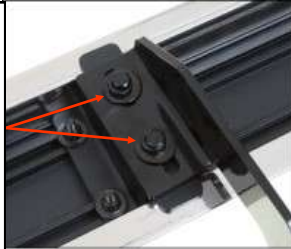
(Fig 9) Step Bar Installed on Bracket Installed (Example)
