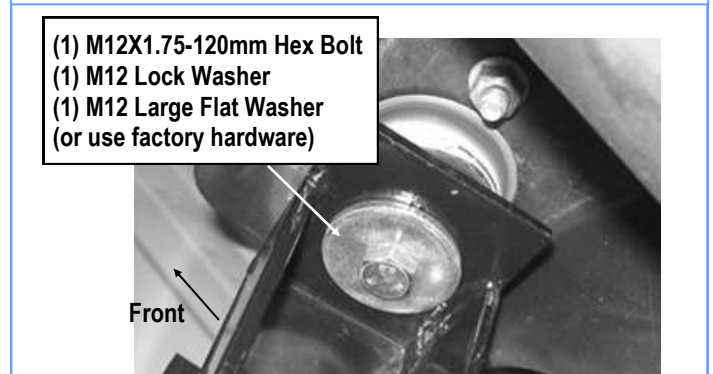
(Fig 1B) Passenger Side Front Mounting Bracket Installed (example only)
