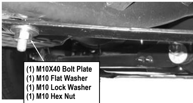
(Fig 3) Passenger Front Support Bracket Installation
