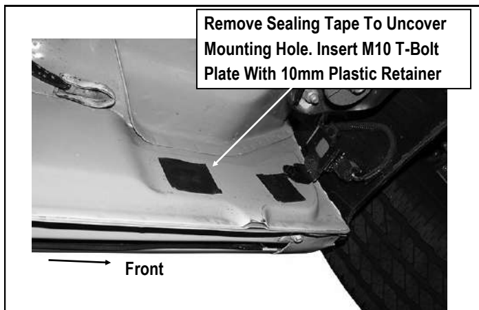
(Fig 1) Driver Front Mounting Bracket Location
