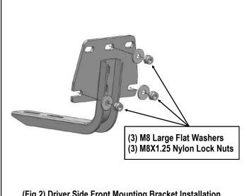
(Fig 2) Driver Side Front Mounting Bracket Installation
