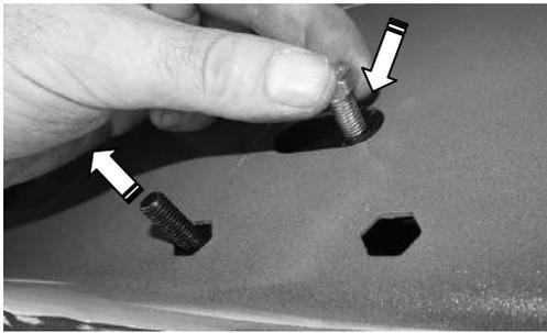
(Fig 4) Use the loose Hex Bolt as a handle. Insert the Bolt Plate into the oval hole and feed the threaded bolt out either factory hex shaped hole. **IMPORTANT:** Do not let go of the hex bolt until after Plastic Washer has been threaded onto bolt (Fig 5).
