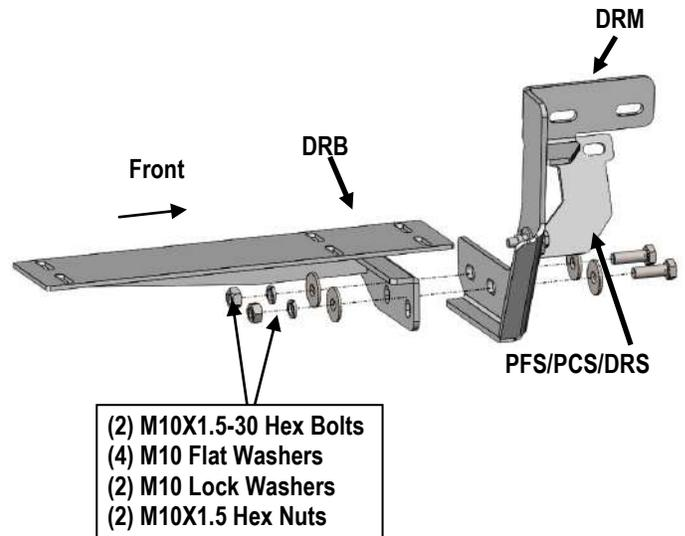
(Fig 15) Driver Side Rear Bar Bracket Assembly
