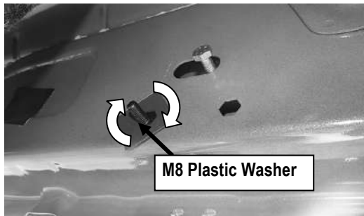
(Fig 5) Thread Plastic Washer onto the welded bolt to hold Bolt Plate in position
