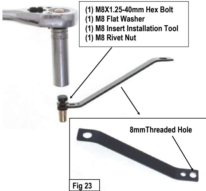
(Fig 22) Assemble Insert Tool As Pictured
