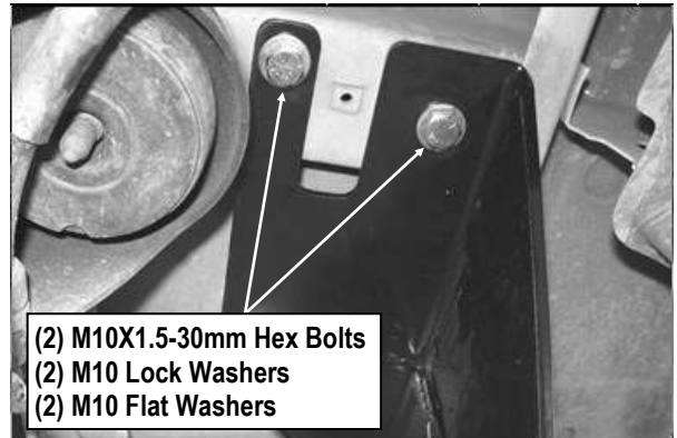
(Fig 3) Driver Side Front Bracket Located
