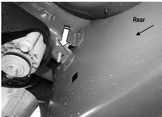
(Fig 8) Insert T-Bolt and folded Washer into oval hole. Thread second Plastic Washer onto T-Bolt
