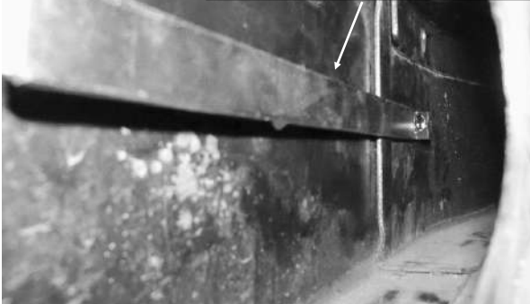
(Fig 3A) Inside View Of M10 Long Bolt Plate Installed (In Driver Side Frame Channel)
