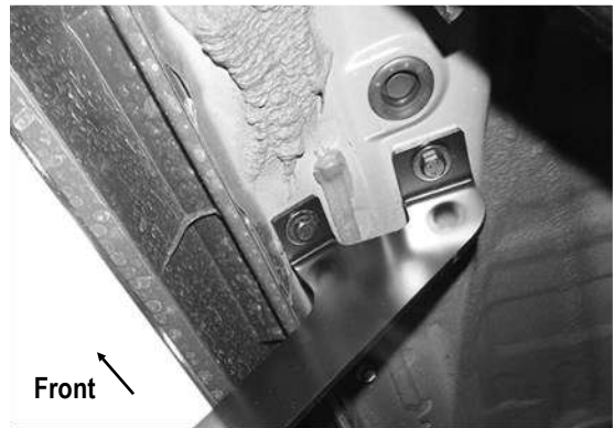
(Fig 3) Passenger Front Mounting Brackets Installed
