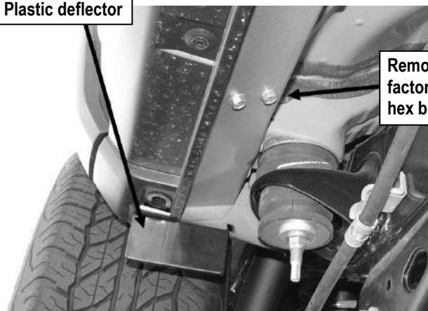
(Fig 3) Passenger Side Rear Mounting Location
