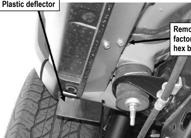
(Fig 3) Passenger Side Rear Mounting Location
