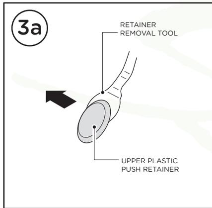
Pull the Plastic Push Retainer out of the rocker panel to expose threaded holes that will be used for bracket installation.
