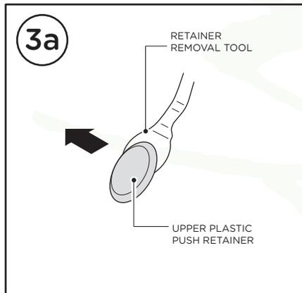
Pull the Plastic Push Retainer out of the rocker panel to expose threaded holes that will be used for bracket installation.
