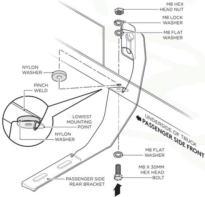
**13.** Fasten the Running Board to the Passenger Side Front/Center Lower Bracket cradles by using (2) M8 Flat Washers, (2) M8 Lock Washers and (2) M8 Hex Head Nuts.
