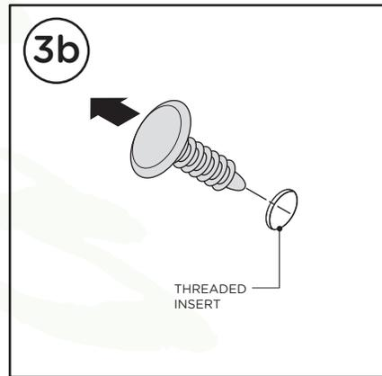
Insert each M8 U-Nut Clip into existing holes in rocker panel, making sure the treads are on the inside of the rocker panel.
