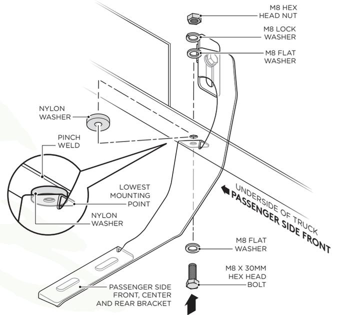
6. Fasten the Running Board to the Passenger Side Front, Center and Rear Bracket cradles by using (2) M8 Flat Washers, (2) M8 Lock Washers and (2) M8 Hex Head Nuts.
