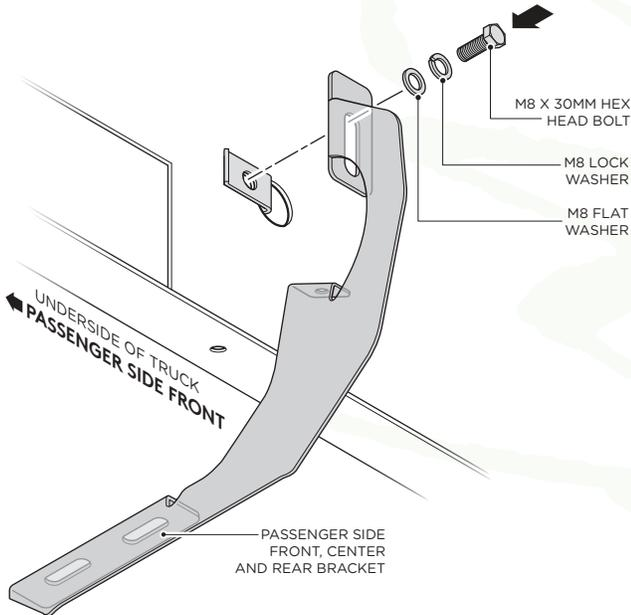
5. Fasten the bottom portion of the Passenger Side Front, Center and Rear Bracket by using (1) M8 x 30MM Hex Head Bolt, (1) M8 Flat Washer and (1) M8 Lock Washer.
