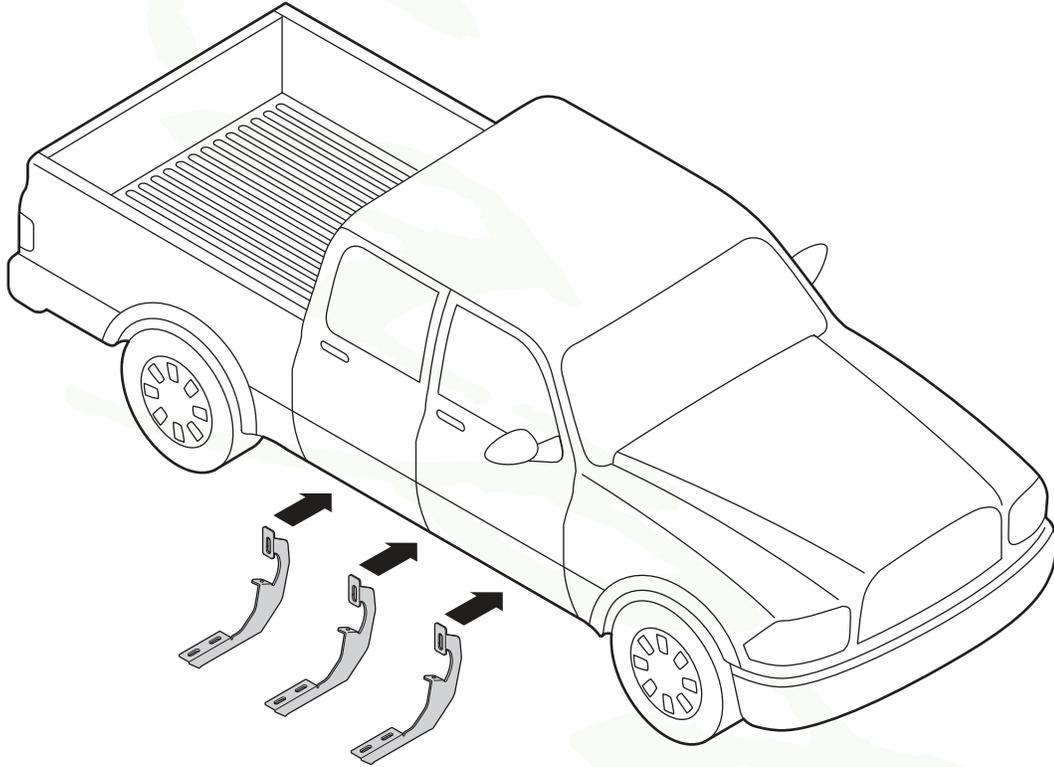
2. Passenger Side Front, Center and Rear Bracket cradles (2a, 2b and 2c) will face towards the rear of the truck.
