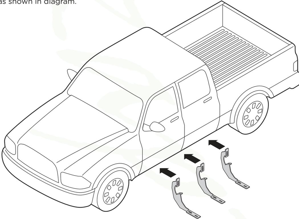
2. Driver Side Front, Center and Rear Bracket cradles (2a, 2b and 2c) will face towards the front of the truck.
