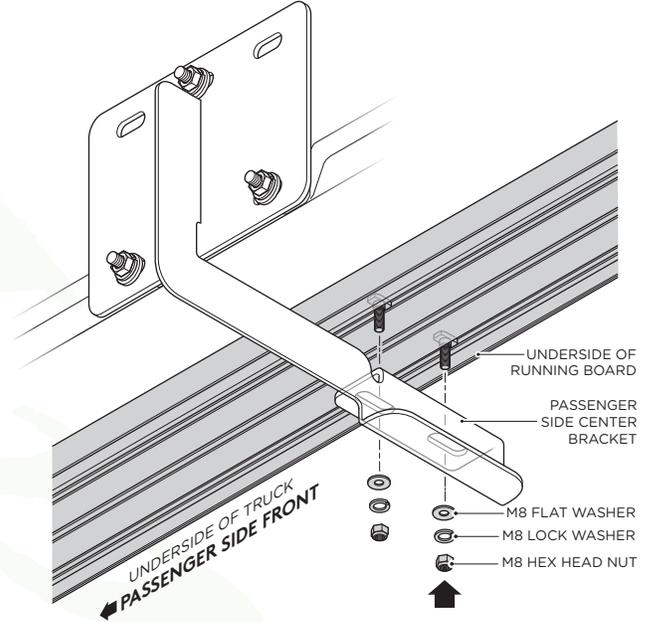
8. Fasten the Running Board to the Passenger Side Rear Bracket cradle by using (2) M8 Flat Washers, (2) M8 Lock Washers and (2) M8 Hex Head Nuts.
