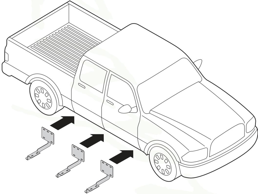
2. Passenger Side Front Bracket cradle (2a), Center Bracket cradle (2b) and Rear Bracket cradle (2c) will face toward the front of the truck.
