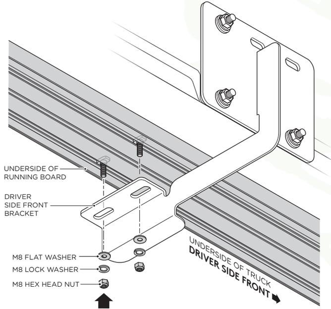
7. Fasten the Running Board to the Driver Side Center Bracket cradle by using (2) M8 Flat Washers, (2) M8 Lock Washers and (2) M8 Hex Head Nuts.
