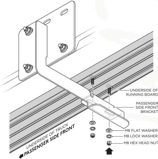
7. Fasten the Running Board to the Passenger Side Center Bracket cradle by using (2) M8 Flat Washers, (2) M8 Lock Washers and (2) M8 Hex Head Nuts.
