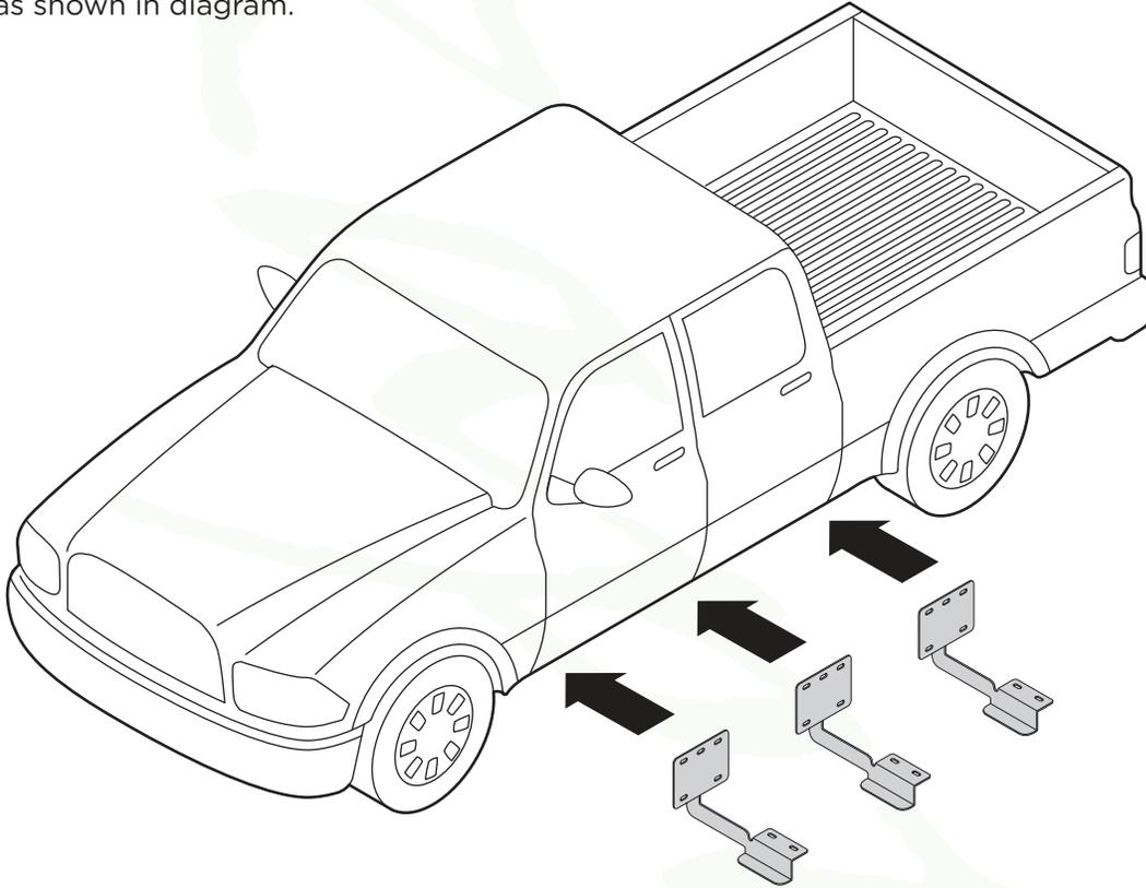
2. Driver Side Front Bracket cradle (2a), Center Bracket cradle (2b) and Rear Bracket cradle (2c) will face toward the rear of the truck.
