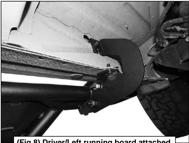
(Fig 8) Driver/Left running board attached to front face of front mounting bracket
