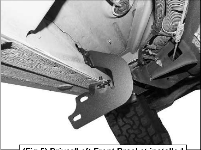
(Fig 5) Driver/Left Front Bracket installed
