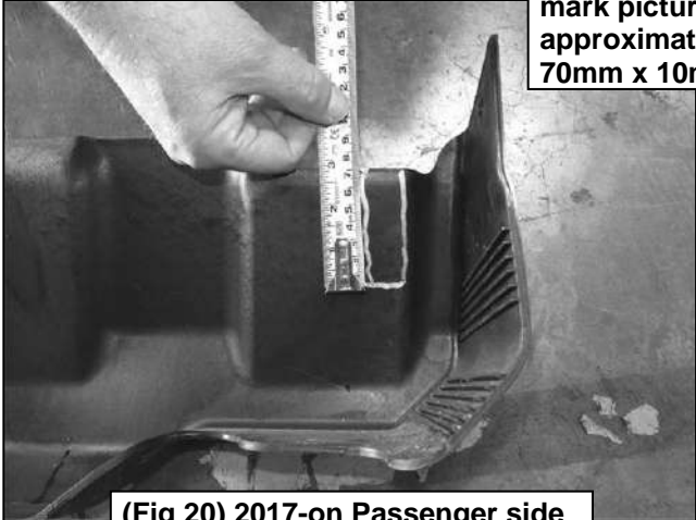
(Fig 20) 2017-on Passenger side DEF cover marked for trimming
