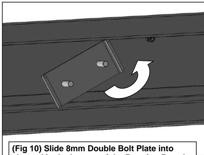
(Fig 10) Slide 8mm Double Bolt Plate into channel in the bottom of the Running Board
