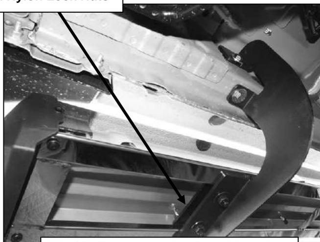
(Fig 12) Passenger side front Mounting Bracket attached to Running Board
