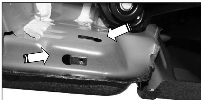
(Fig 8) Passenger side rear mounting location
