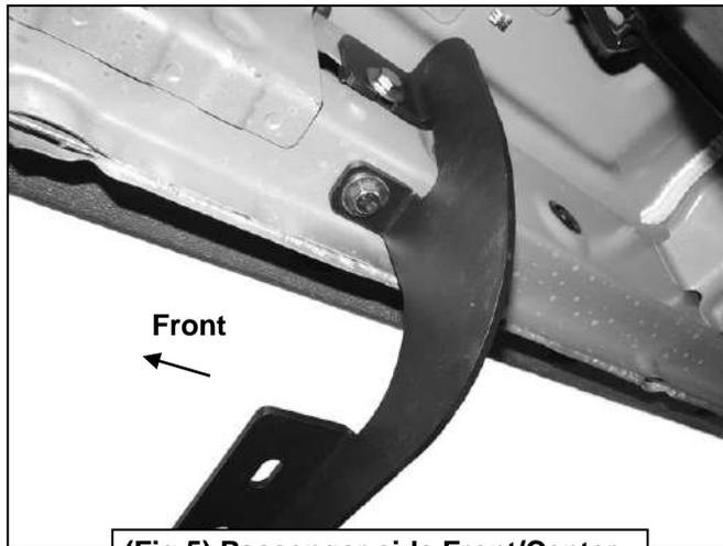
(Fig 5) Passenger side Front/Center Mounting Bracket installed
