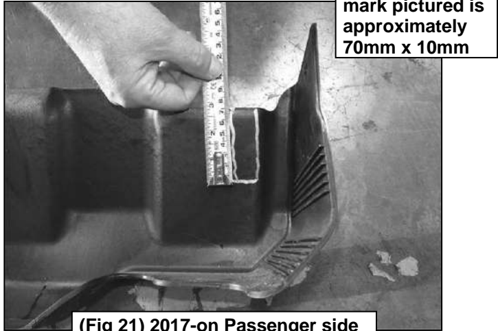
(Fig 21) 2017-on Passenger side DEF cover marked for trimming
