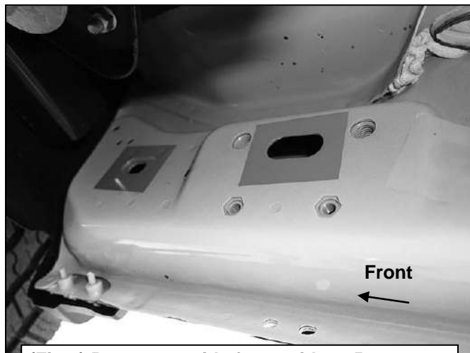
(Fig 8) Passenger side front mid 2015-on, models with factory installed threaded inserts
