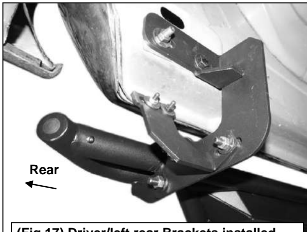
(Fig 17) Driver/left rear Brackets installed
