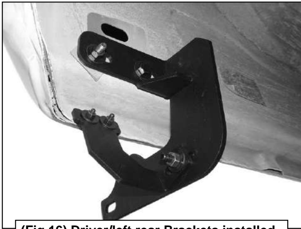
(Fig 16) Driver/left rear Brackets installed
